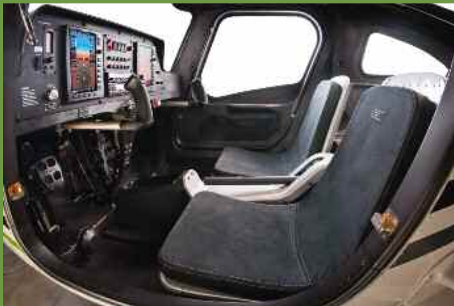
Manual flap lever, fixed seats, upward opening doors and unusual control sticks. Note enlarged window in right door
