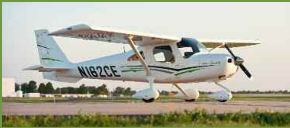
Dorsal fin aids spin recovery. Note how the wing strut doesn't obstruct the door, important in flying schools
