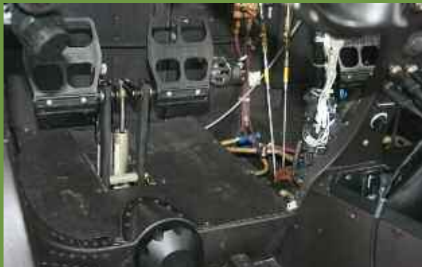
Pedals are strong and easily adjusted with a knurled wheel. Toe brakes have good geometry
