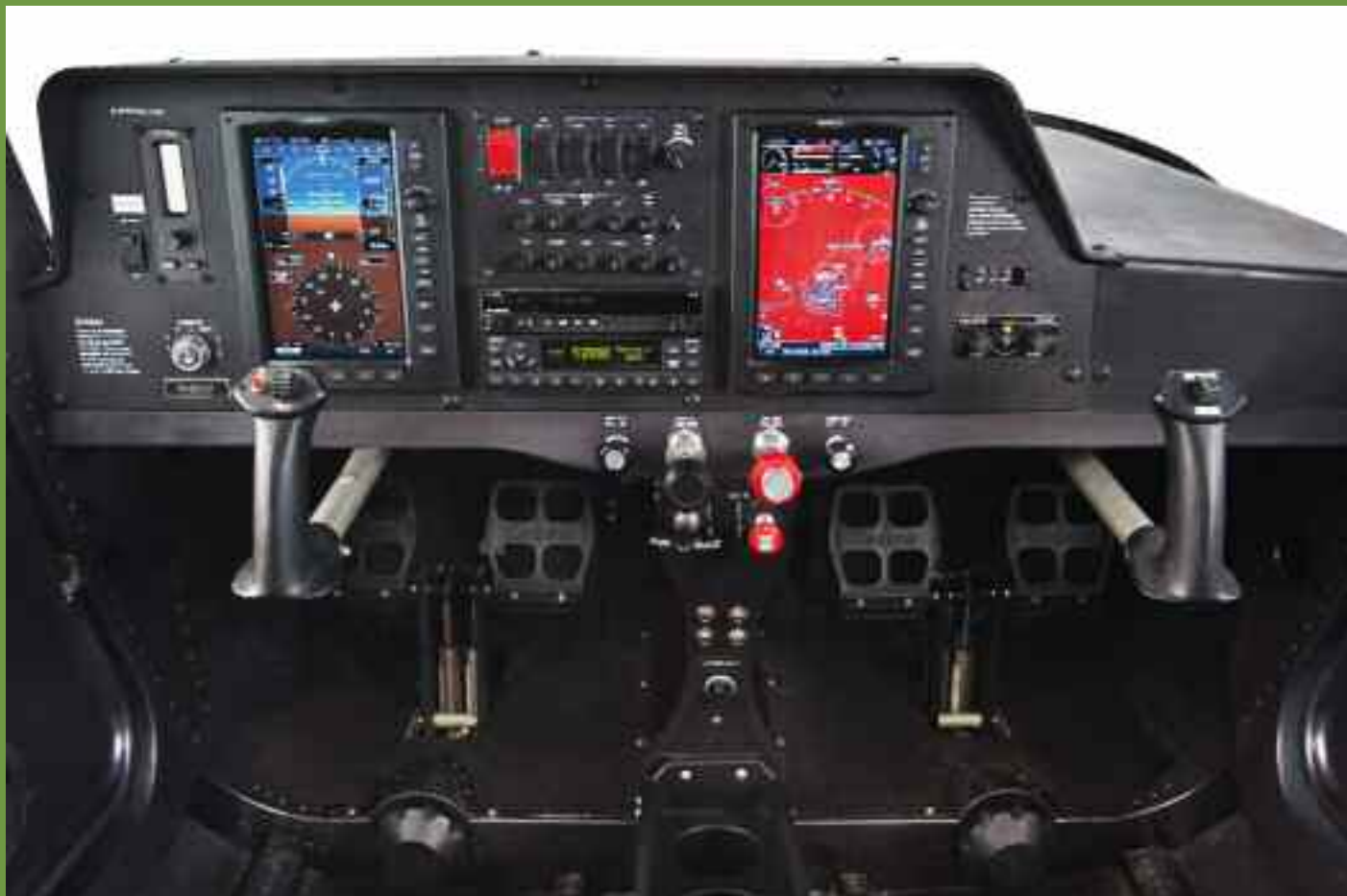
The right screen is optional (like the PLB and parachute), but early indications are that most customers will take it. Having two screens gives redundancy should one fail
