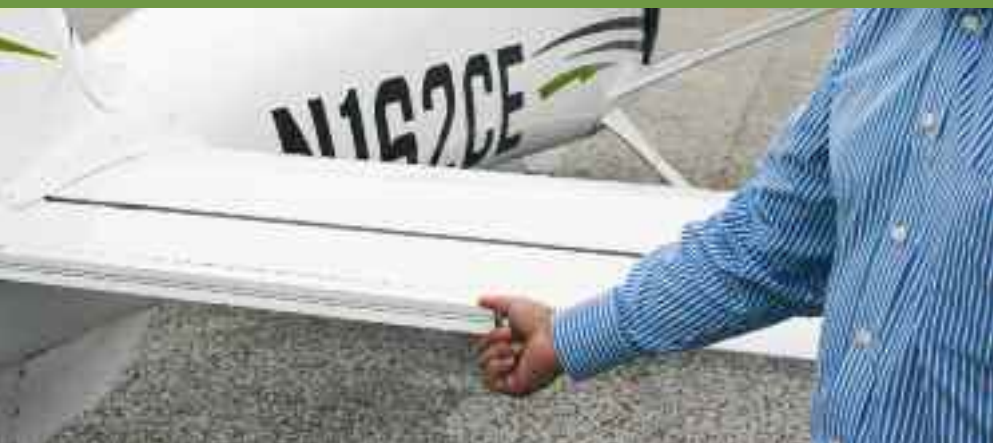
'T' addition to trim tab reduces elevator lightness for smoother landings. Later models might have a neater solution
