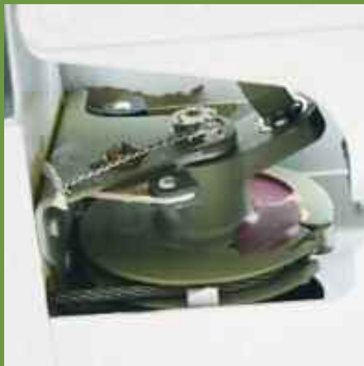
Control cable is fixed to this pulley wheel which deflects the aileron
