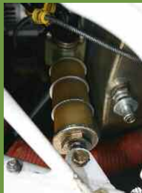
Sturdy and well-designed nosewheel suspension
