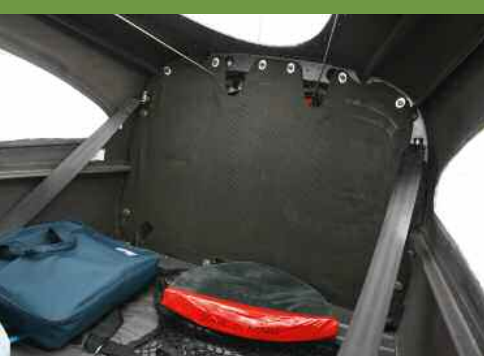
Generous luggage bay behind seats. Note lightweight access 'panel' and extra cushion for short occupants
